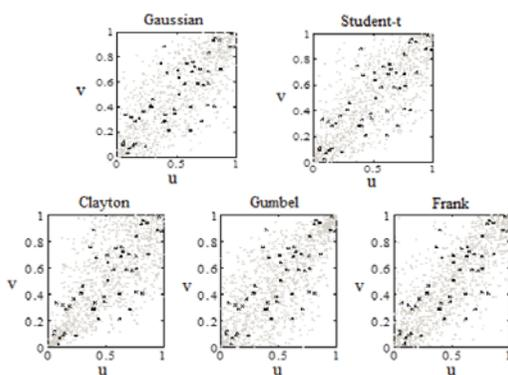
FIGURE 4. Simulated random sample of size 1000 from the five selected copulas with parameters estimated by the method of IFM using the precipitation-runoff volume data, whose pairs of ranks are indicated by an "X".
