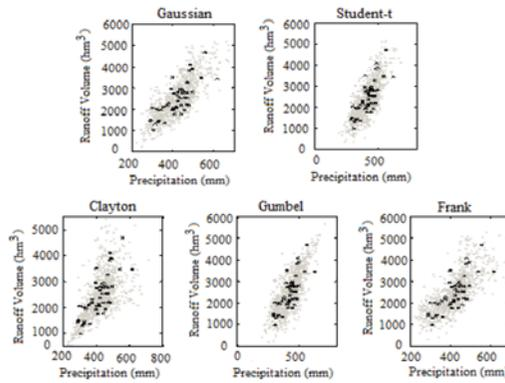
FIGURE 5. Same data as in Fig.4, upon transformation of the marginal distributions as per the selected models for the precipitation and the runoff volume data, whose pairs of observations are indicated by an "X"
